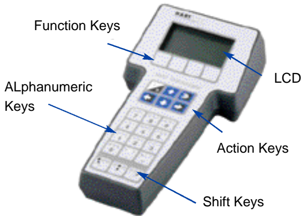
Figure 2. The HART Communicator provides features that make the communicator fast to learn and easy to use.
